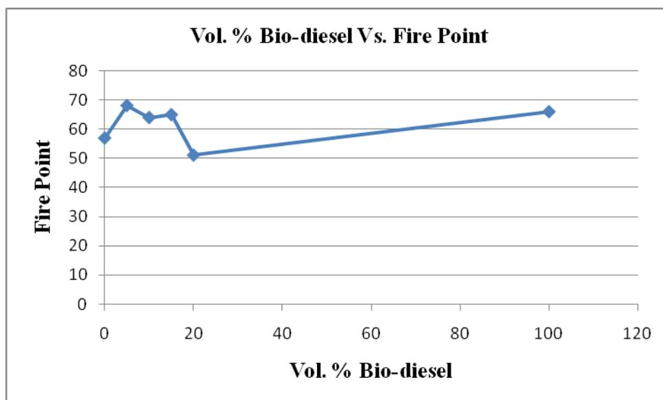
Discussion: Both flash and fire points are slightly increased when petro diesel is blended with 5%, 10%, 15% and 20% bio diesel. However the increase is very minimal, it is not consider as disadvantage. It can be also conclude that slight increase in flash points reduces the inflammability petro diesel.
